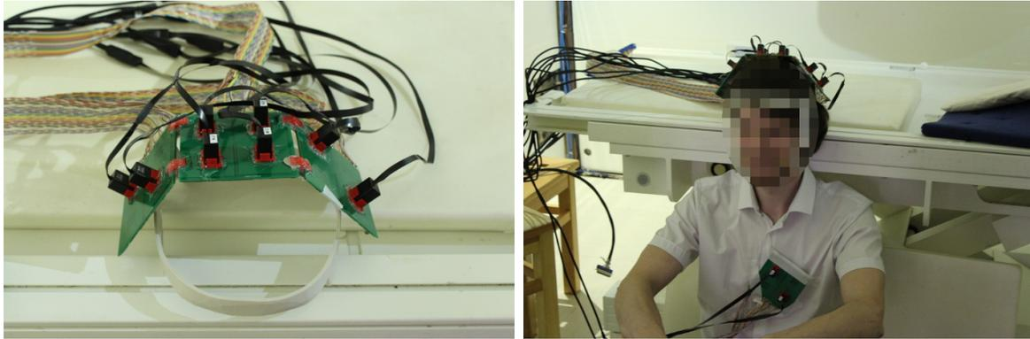
Figure 9.1: Setup for proof of principle quantitative imaging of MNP in a glioblastoma. The setup consists of 48 excitation coils and 16 OPM channels. Four additional OPM channels are used to measure MCG simultaneously. The coil board on the chest is solely used for mounting the OPM.
